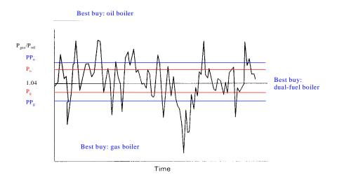
$P_{\rm o}$  is the fuel price ratio at which the dual burner should be switched to oil when the relative price of gas is going up;  $P_{\rm g}$  is the ratio at which the dual burner should be switched to gas when the relative price of gas is going down. The gap between  $P_{\rm o}$  and  $P_{\rm g}$  increases with the cost of switching and with volatility.
